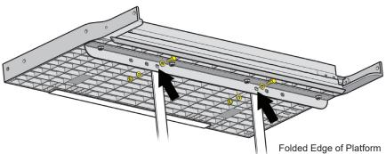
Loosely fasten the footplate to the vertical support bracket using (2) <u>M10 x 35 Hex.</u> <u>Head Bolts</u>, (4) <u>Flat Washers</u> and (2) <u>Nylock Nuts</u> (Bag #3).
