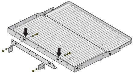
Loosely install the seat platform sub-assembly to the front seat back support brackets using (4) <u>M8 x 55 Hex Head Bolts</u>, (8) <u>Flat Washers</u> and (4) <u>Nylock Nuts</u> (Bag #2).
