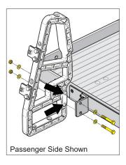
6. With the platform folded, loosely install the seat platform to the vertical support bracket using (2) <u>M10 x 25 Hex Head Bolts</u>, (4) <u>Flat Washers</u> and (2) <u>Nylock Nuts</u> (**Bag #2**).
