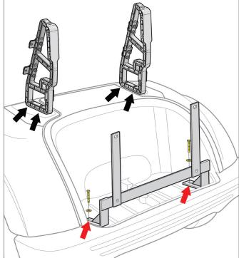
Install the sub-assembly brackets and the platform support bracket to the platform using using (2) <u>M10 x 35 Hex Head Bolts</u>, (4) <u>Flat Washers</u> and (2) <u>Nylock Nuts</u> (**Bag** #2). Hand tighten enough so the brackets are snug but still adjustable.
