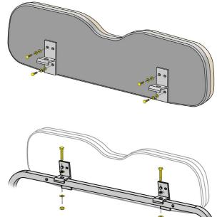
back assembly to the rear seat back support frame using (2) <u>M10 x 45 Hex</u> <u>Head Bolts</u>, (4) <u>Flat</u> <u>Washers</u> and (2) <u>Ny-</u> <u>lock Nuts</u> (**Bag #5**).
