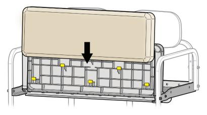
Fasten the handle to the seat platform using (2) <u>M6 x 20 Phillips Head</u> <u>Countersunk Screws</u> (**Bag #5**). Hand tighten to lock the seat bottom into place.
